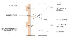
Face nail through center of batten and siding.
