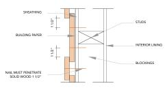
Face nail through center of batten and double nail siding.
